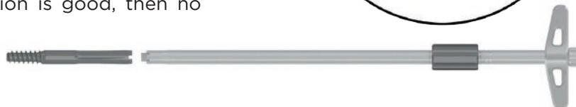
Three circles exist beside the black thumbwheel, respectively standing for 0mm, 5mm, and 8mm compression distance. Take 5mm compression as example. Screw the thumbwheel to the 5mm circle position. After totally inserting the Femoral Compression Screw B, then rotate the thumbwheel clockwise until the black thumbwheel flush with 0mm line. The longest compression distance is 8mm. More than 8mm compression may cause fracture bone collapse.
