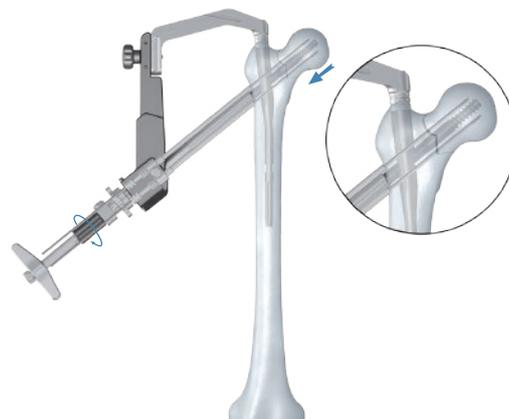
After inserting screw, the handle of Screwdriver (13031024) should be 0° or 90° perpendicular to the Proximal Aiming Device, 135° (13031007). So that the Fastening Screw would be able to sit exactly on one of the four grooves of the Femoral Compression Screw.
